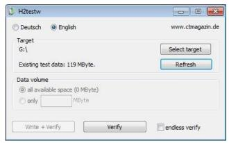
With this software you can verify the capacity and ensure that it works well. The speed measured however depends on both the stick or card and the host device. The tiny capacity of the device in this example resulted in a test time of about a minute; expect much longer times for modern multi-Gbyte devices. Nevertheless, it's worth taking the time to check a new SD card before trying to use it in your camera on a trip to Europe. Go to Page 1
