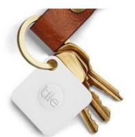
device about 1-inch square and ¼ inch thick. Here's how it works. I attached a Tile to my key ring. The app in my phone can see the keys and keeps track of their location. When I can't find my keys, I can make the Tile ring from my phone if it is within 100 feet. If I have my keys and have misplaced my phone, I can make my phone ring from the tile on my keys even when it is on silent. I use the ringing feature a lot.
